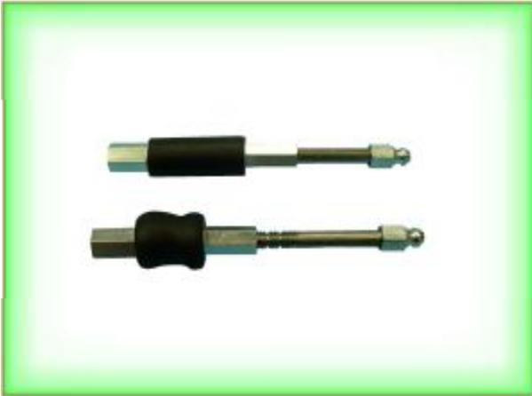
It is a special system, which enables to dismount the packer immediately after the grouting. The fixation of the packer into the bored hole is carried out by means of the socket wrench M9. After tightening of the packer in the bored hole, two recesses behind the nut are uncovered which enable an easy break of the grouting packer.
