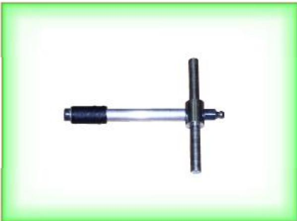
The packer is fitted with tightening fly nut.
