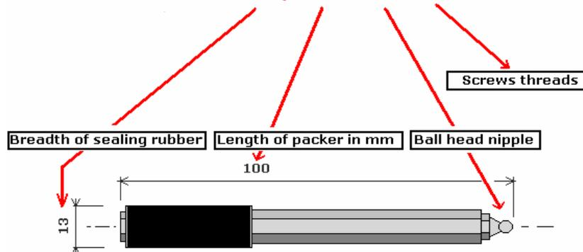
Packers are fitted with the nipple, which ensures the clack-valve function. The connection of the OPK packer onto the grouting pump hose is done by means of the coupler. The diameters of the sealing rubber are from 10 mm to 17 mm. The lengths of the OPK are from 70 mm to 500 mm.
