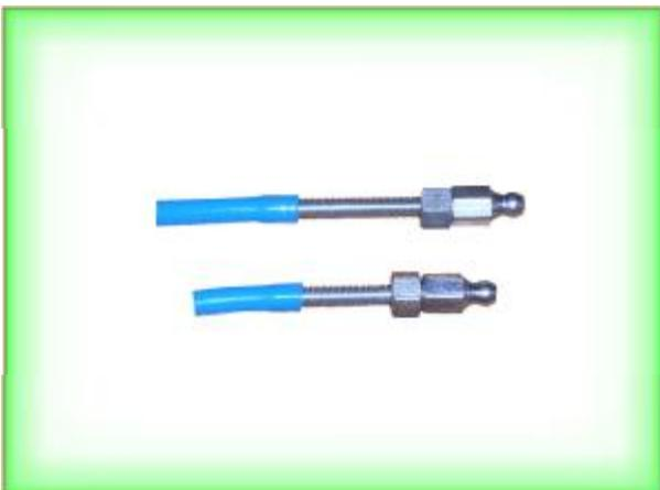
It is a special packer determined for low-pressure grouting, i.e. into the joints between the tiles. The bored hole diameter is 6 mm for this packer. **Recommended working pressure is :** to 5 Mpa (50 bars).
