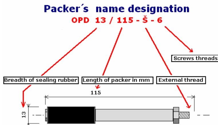
The connection onto the grouting pump hose is carried out directly onto the mixing gun with the bored thread of an appropriate size. The diameters of the sealing rubbers are from 8 mm to 19 mm. The OPD lengths are selected optimally according to the massif, into which they will be placed into from 70 mm to 500 mm.
