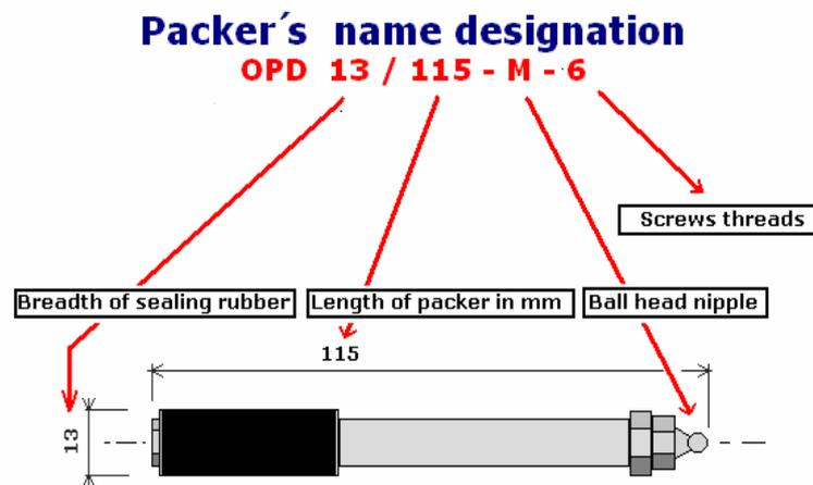
*or with a screw M5, M6, M8 or M10 according to a version without any clack-valve.*
