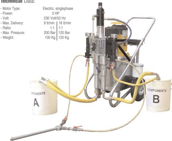
HTP 21000 BICOMPONENT is an airless hydraulic piston pump ideal for bi-component products with mixing 50:50.
